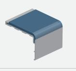
XT stair edgings offer the ultimate solution in reducing slips, trips and falls on stairs and comprises aluminium channels with a choice of inserts. The insert extends around the leading edge of the stair edging to ensure that foot contact is always made with the slip-resistant element of the stair edging.
